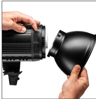
2. Place the reflector in the accessory holder and lock the reflector in place. lock the reflector in place with a clockwise rotation.
